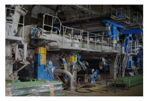
7.4 Press section Press section includes 3 nips in combination with Kusters S-rolls 1st nip: suction roll ©1050 mm and S-roll ©620 mm 2nd nip: suction roll ©1050 mm and press roll ©1250 mm 3rd nip: press roll ©1250 mm and S-roll ©620 mm
