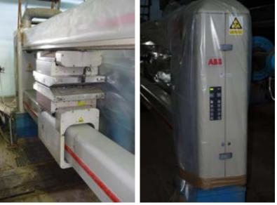
7.8 <u>Pope reel</u> The carrier drum of the reel is ⊚1000 mm x 4670 mm. This section is equipped with Turn-up System, manufactured by IBS.
