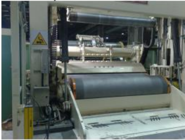
New rewinder By Vas installed in 2008
