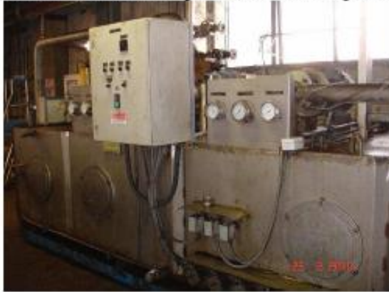
Nr. 2 Automatic lubricating unit for the lubricating of the machine
