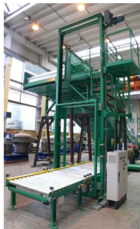
Conveyer back part - roller-type line
