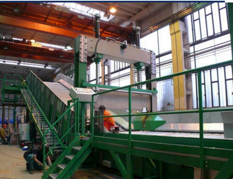
Completion of a chain conveyer with steel plates and a waste reels splitter for the Russian customer
