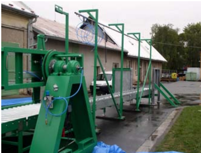
Console for pneumatic wire cutting
