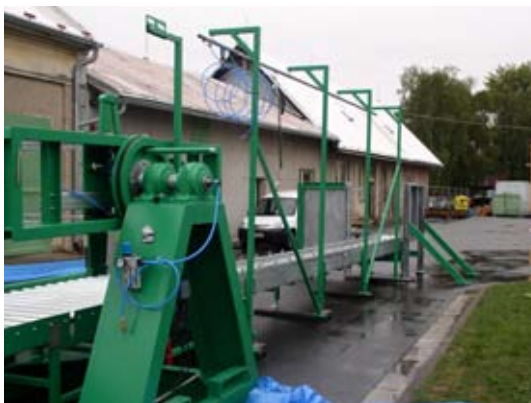
Ingoing chain conveyer with pneumatic unwiring
