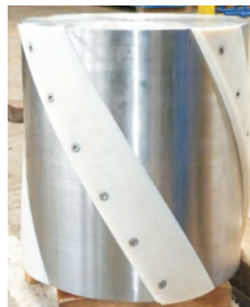
Prototype of STU-081 rotor with plastic vanes
