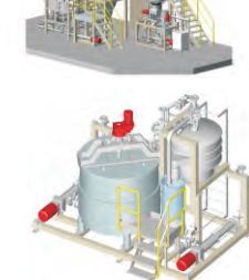
Size press and film press workstations
