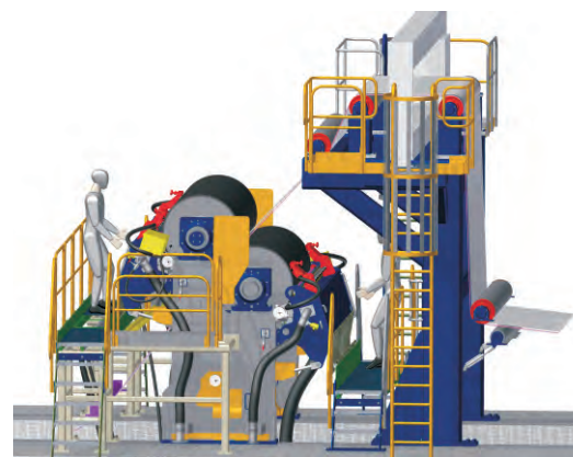
Size press and film press workstations
