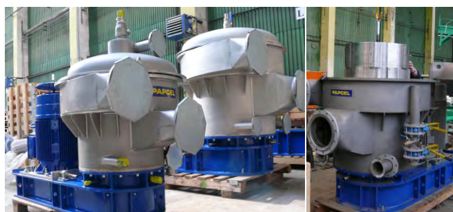
STU-081-L with its cover for efficient stock venting intended for fine screening of light impurities; STU-201; rotor installation
