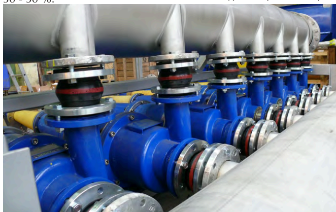
Details of spiral inlet parts, station of cleaners SVO-25 intended for Egyptian customer
