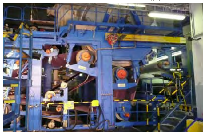
Press section + drying section (Yankee cylinder diameter 4 000 mm)
